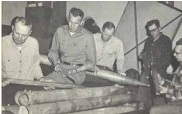
LM volunteers cleaning pipes from the old Möller after they were damaged by water infiltration.
